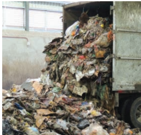
Commercial organics that have been processed by Republic Services at its MRF on Newby Island arrive in walking floor trailers and are directly loaded into the digesters.
